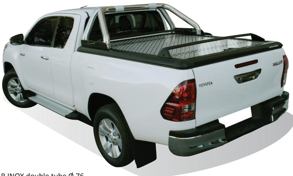
ROLL BAR INOX double tube Ø 76
