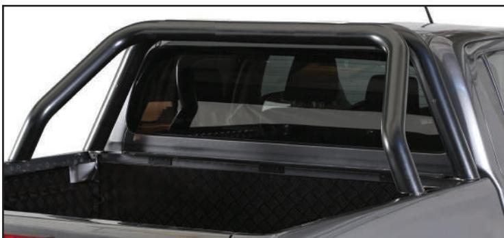
ROLL BAR INOX double tube  $\varnothing$  76 mm
