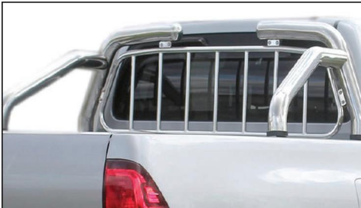
ROLL BAR INOX double tube  $\varnothing$  76 mm
